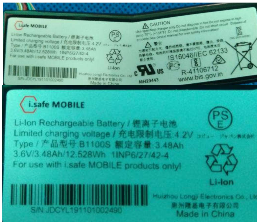
电池组铭牌 View of the battery nameplate
